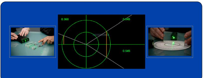
A web based app is used to collect data with real lasers so that students can uncover the laws of reflection and refraction by observing patterns.
