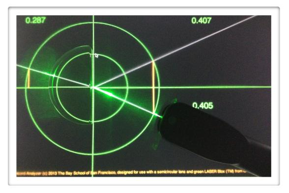
5.If the room lights are low enough, you should be able to see the reflected beam quite easily in the upper right hand quadrant. Move the gray line in that quadrant so it is directly below the reflected beam. Finally, move the gray line in the upper-left hand quadrant so it is directly below the beam that passes through the lens (**the transmitted beam**).
